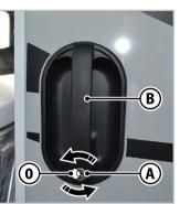
*Fig.5.1 - Opening/closing the entrance door from the outside*
