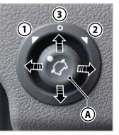
Fig. 3.1 - Adjusting the mirrors
