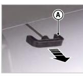
Fig.6.35 - Grey water drain valve
